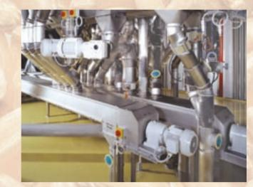
Semolina collection screw conveyors of special steel for maximum sanitation
